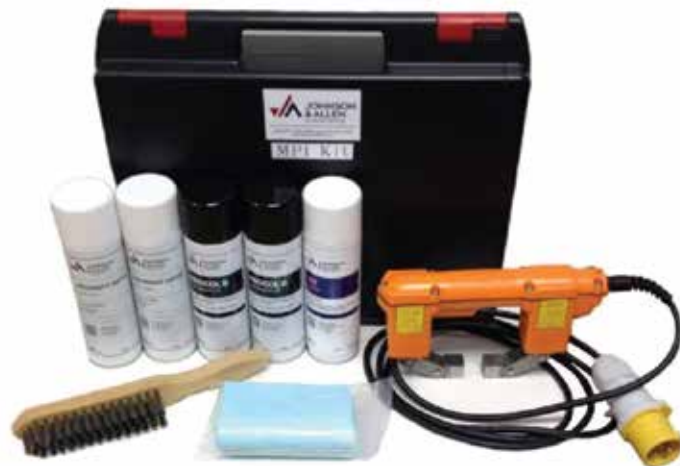
Electrical magnetic particle
